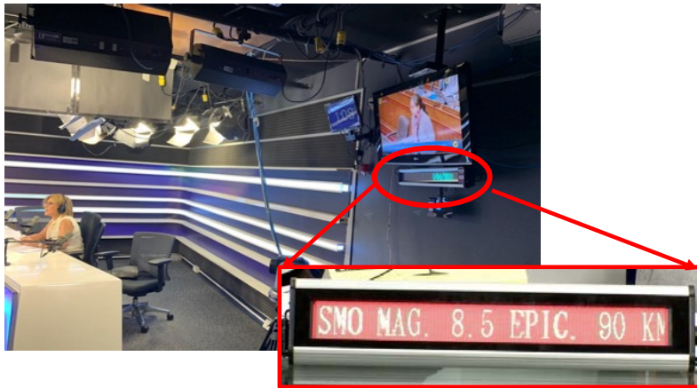
EWBS display in operation at a radio station in Lima, Peru
